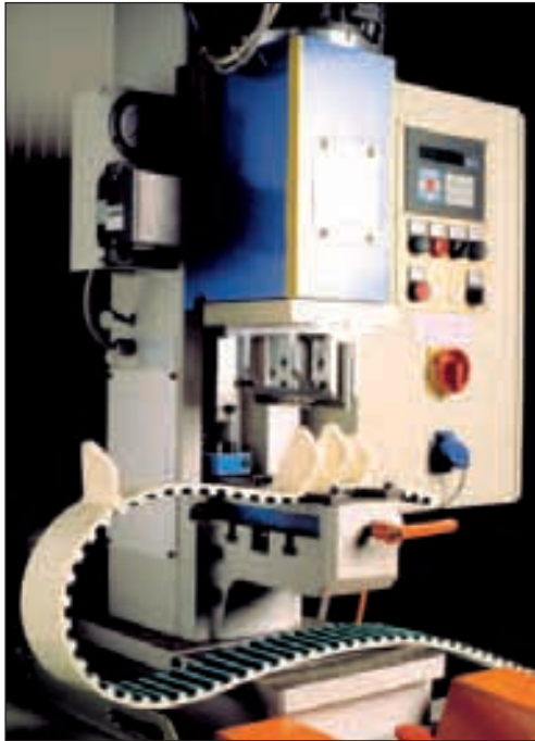
Cleat welding machine
