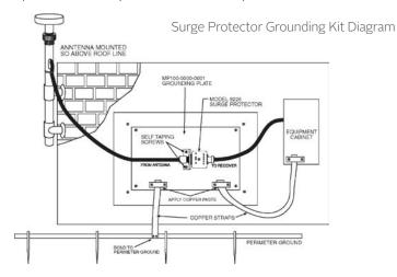
Spectracom offers a Surge Protector Grounding Kit, Model 8226-0002-0600, that serves as a single point ground connection for the GPS Antenna Surge Protector, equipment rack, GPS receiver, and other surge protection devices to a perimeter ground system. A single point ground system is recommended to provide protection from lighting strikes.
