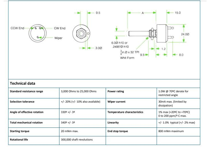
General purpose conductive polymer panel control of robust and reliable construction. Glass filled nylon body moulding; beryllium copper contact; brass spindle and bush; silver plated brass tags.
