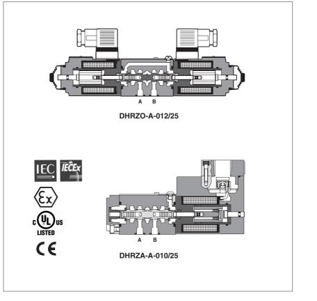
DHRZ\* are 3 way, proportional pressure reducing valves, direct operated, with standard ISO 4401 size 06 mounting surface
