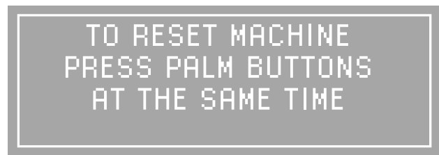
Figure 13-6 Startup Fault Display
