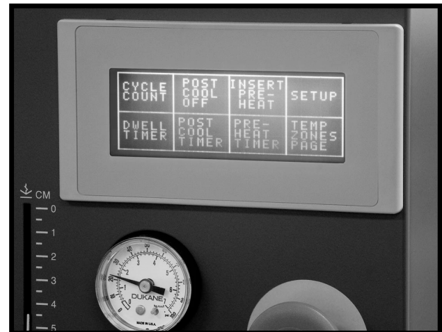
Figure 5-3 Main Control Panel and Touch Screen Display
