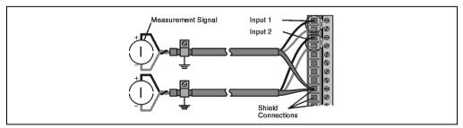
Figure 126: AI775 signal cable connection
