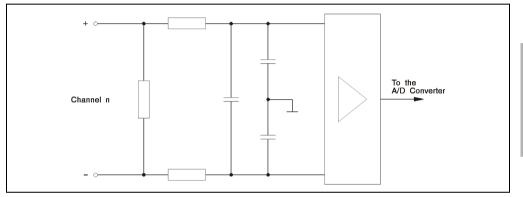
Figure 128: AI775 input circuit diagram
