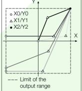
Fig. 4. Examples of settings with linear characteristic.
