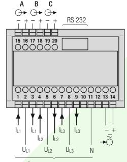
Measuring inputs, acc. to measuring mode
