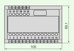
Fig. 6. SINEAX M 563 in housing P20/105 clipped onto a top-hat rail (35 x 15 mm or 35x75 mm, acc. to EN 50 022).
