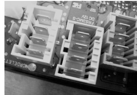
new Fusebox with connectors 'RAST5'
