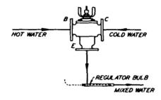
Fig. I - Illustrated is a simple means for mixing hot and cold water where a rough mixing is suitable.
