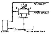
Fit. 3 - Illustrated is a method of controlling the cooling of engine lubricating oil.
