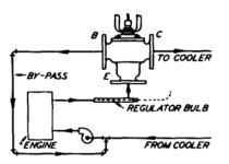
Fig. 2 - Illustrated is the most widely used method of cooling water control for internal combustion engines.
